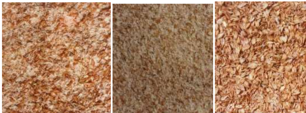
Figure 5.4 P. ovata seed after it had passed through the rice huller. Then separated into husk and crushed seed by an air leg separator. (McNeil, 1985)
